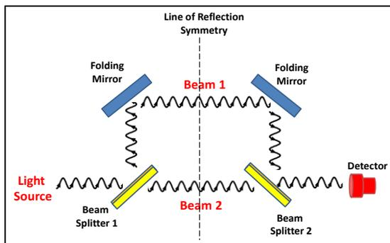
Figure 5: Mach Zehnder interferometer
