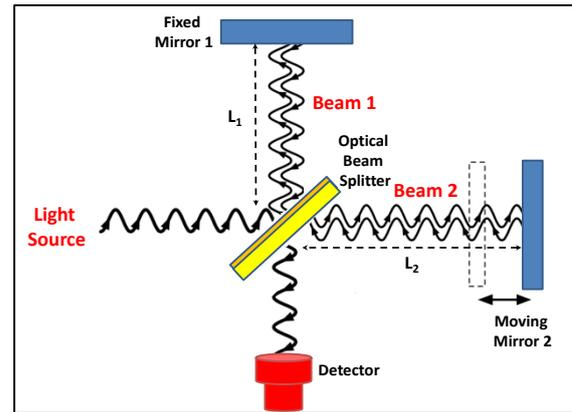
Figure 1 : Scanning FTIR interferometer
