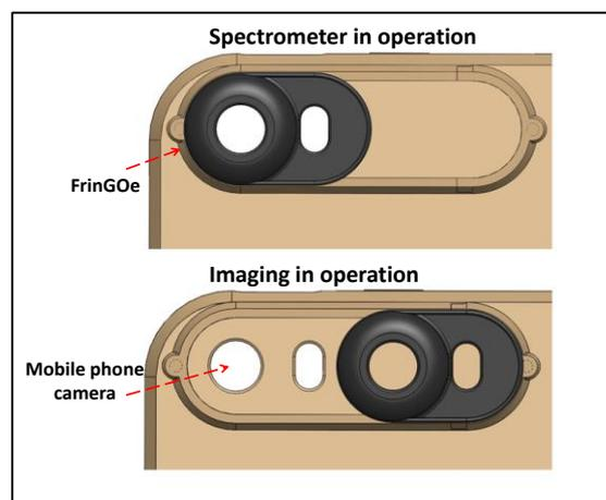
**Figure 11: FrinGOe switchable between spectroscopic and imaging mode**
